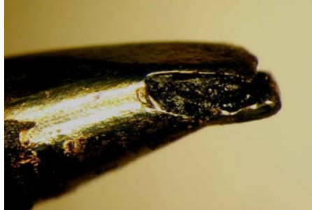
Lead-free tip failure after 3 weeks
